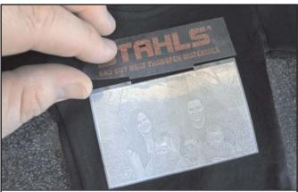
4. Place the laser cut notch in the carrier (backing) together then heat apply both colors at the same time.
