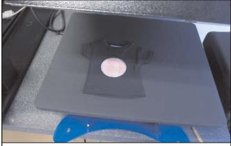
5. Remove the engraved material from laser. Turn it over, engaving face down, and place on the garment. Then heat press using suggested Stahls' settings. Remove from heat press and hot/warm peel.
