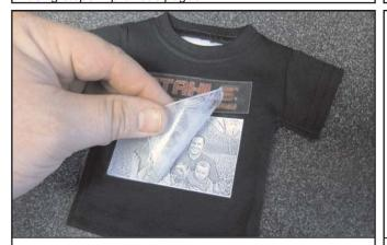
5. Heat apply both colors at the same time, then warm peel the carrier (backing).
