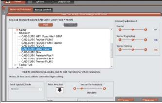
2. Print file to ULS laser system, select Stahls' material from the ULS database. Then select "Fabric/Stahls." Next select desired material.
