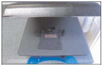
5. Heat apply then warm peel the carrier (backing).
