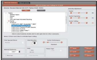
4. Print file to Universal laser system, and select Stahls' material from the ULS database. Choose "Fabric/Stahls" and select desired material.
