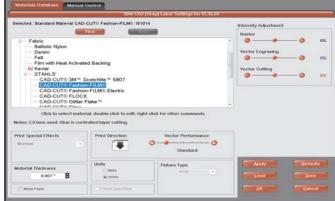
2. Print file to ULS laser system. Select Stahls' material from the ULS database by choosing "Fabric/Stahls." Then select the desired material.
