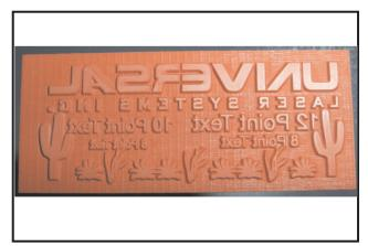
**6.** Engrave rubber stamp. (Air assist with air cone is recommended) Cut out the stamp with laser or scissors. Clean finished rubber stamp ("Simple Green" cleaner works best) and place onto stamp.
