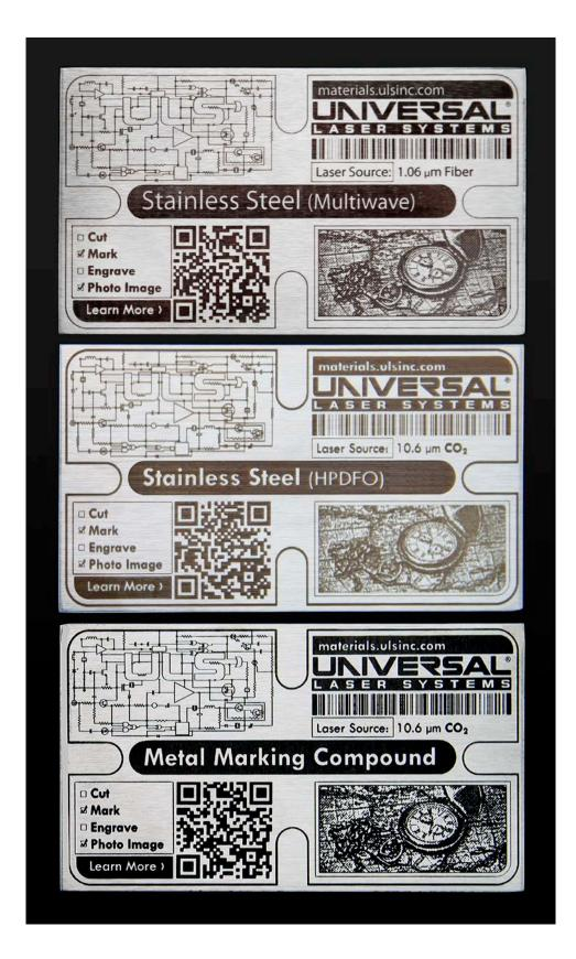
This image is a side-by-side comparison of the three marking methods, beginning at the top with direct marking with the fiber laser, then direct marking with HPDFO and a  $CO_2$  laser, and finally metal marking compound with a  $CO_2$  laser.
