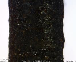
Figure 3: Micrograph of a laser cut polycarbonate edge using the typical method
