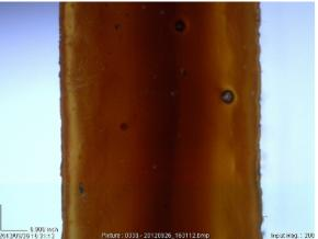
Figure 5: Micrograph of laser cut polycarbonate edge using the Smooth Edge Method
