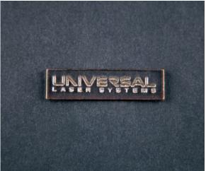
Figure 2: CO<sub>2</sub> laser marked sample
