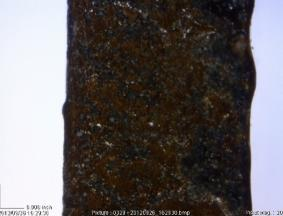
Figure 4: Micrograph of a laser cut polycarbonate edge using the Multi-Pass Method
