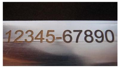
It is possible to engrave into the surface of metal using the fiber laser. It is a slower process than marking and requires iterative passes to achieve depth. While it is possible to achieve greater depth with additional engraving iterations, the best results exist around 0.003" to 0.005" into the material. To create this depth, install the 2.0 lens to provide sufficient energy density for
