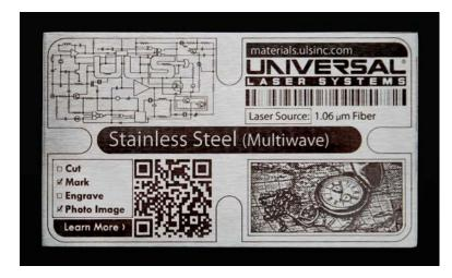
Creating a surface mark on metal is very straight-forward using the fiber laser. Lens selection will vary depending on the metal you plan to work with as well as any focal tolerance or focal distance considerations due to part geometry. Typically the 4.0 lens produces the best results on steel and titanium, while the 2.0 lens will work well for most other metals. The focal tolerance for the 2.0 lens is +/- 0.02" while the tolerance for the 4.0 lens is +/-
