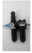
Multi-Stage Air Filtration Unit offers a media stage and a coalescing filter stage to ensure air coming from the air compressor is free from debris prior to entering the laser system. These units are configured with a regulator and hose to the laser system as well. Note: Operators that plan to cut
