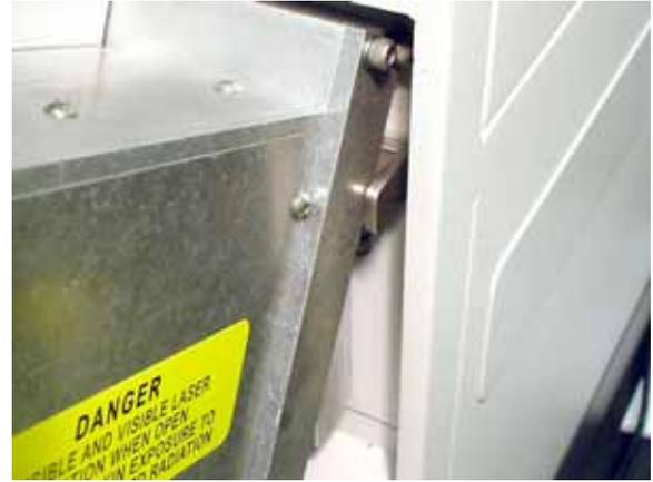
Slowly rotate the Laser Cartridge making sure that the Alignment Plate is centered in the small gap of the Alignment Fork. Keep rotating the laser until the Laser Latch “clicks” and locks the cartridge into place. **Make sure that you do not pinch any wires during this process.** It may require some slight force to actuate the latch.
