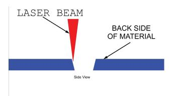
The convergence of the laser beam will produce an angled cut on the Braille text as shown left. The angle cut is critical for keeping the Raster beads in place.
