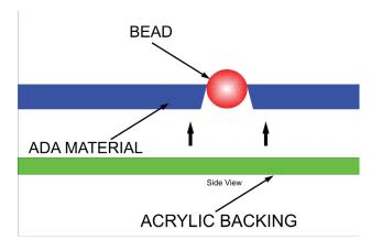
In this illustration you can see how the angle cut keeps the Raster beads in place.
