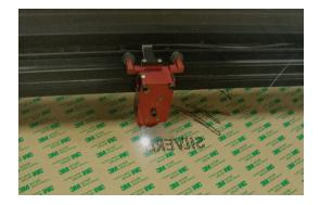
Tip: We recommend you make two passes at half-power when cutting Rowmark ADA Alternative® plastic. It is critical to avoid "melt back" when vector-cutting the Braille characters so that the acrylic or stainless steel Raster beads fit tightly (see below). This will be explained in more detail later.
