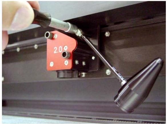
Using a 3/16 socket tool or 5mm wrench, attach the needle valve to the port where you removed the plug. Be careful not to cross-thread the small device when installing and do not over tighten it.
