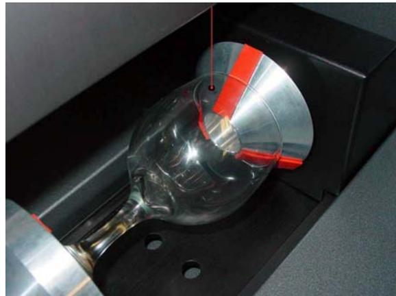
Continue repositioning until the Red Dot is on top of your mark. When it is aligned, in the VCP, locate the X-axis coordinate number. Either write this number down or remember it. This is the coordinate of the Red Dot pointer and it is also where you will need to position your graphic. Ignore all other coordinates.
