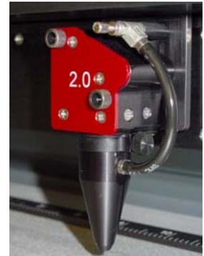
The cone attaches to the base of the Focus Carriage and will force air directly onto the surface of your material to reduce the burning effects of the material from the laser beams intense heat. It also helps disperse the smoke and gases that are created from the processing of materials. It contains a needle-valve assembly to control airflow through the cone.
