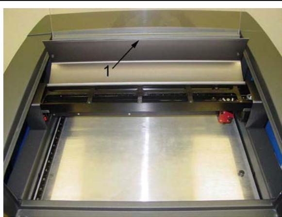
1. Rotate the cover up and over the top of the X-axis Arm. The cover is held down by magnets so it may “stick” slightly when you first begin to pull it forward.
