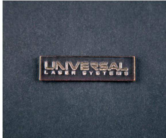
Figure 2: CO<sub>2</sub> laser marked sample
